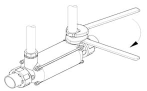
To prevent the stainless steel fitting from detaching itself from the heat exchanger housing and, as a result, also from the corrugated coil, and to prevent leaks from occurring, the stainless steel fitting should be firmly tightened with a second spanner or pliers. (See ilustration)
